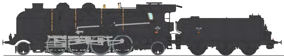
6-141 E 458 SNCF Veynes railways depot - double smokestack, large smoke deflectors, DABEG water pump, 25m 3 25A88 tender SNCF 6-141 E 458 Veynes - Doppelschornstein, großen Windleitblechen, DABEG Pumpe, 25 m 3 25 A 88 Tender
