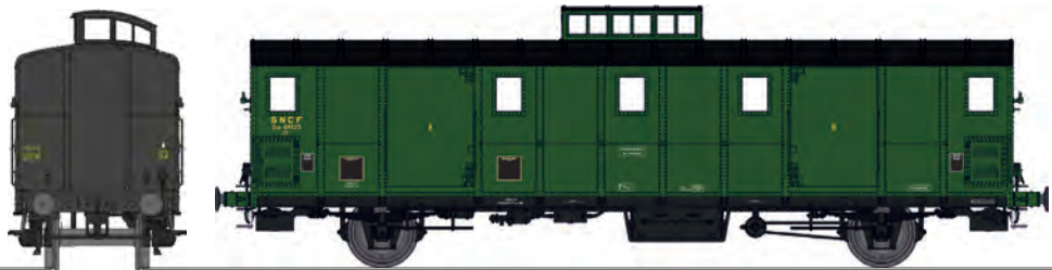
Black riveted roof, P.O. lookout box, pillow block bearings, Fenced windows Ex-P.O. "Toulouse" N°49523 Era III Dach genietet schwarz, PO Dachkanzel, Gleitachslager, «Toulouse» Ehem. PO Fenstergitter, N°49523 Ep.III
