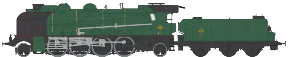
5-141 E 284 SNCF Villeneuve railways depot - double smokestack, large smoke deflectors, ACFI water pump, 25 m 3 25 A 27 tender SNCF 5-141 E 284 Villeneuve - Doppelschornstein, großen Windleitblechen, ACFI Pumpe, 25 m 3 25 A 27 Tender
